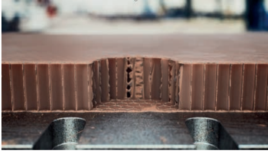
Position substrate material with the prepared hole.
